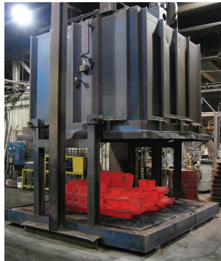
Quaker City Castings can heat treat castings up to 1,900°F.
