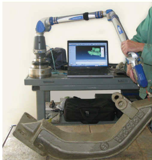
Dimensional accuracy measured with the FARO Edge.
