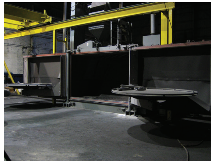
Our double door table blast allows quick and efficient processing of castings.
