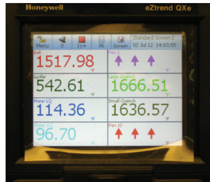
Computerized monitoring of heat treat cycle.
