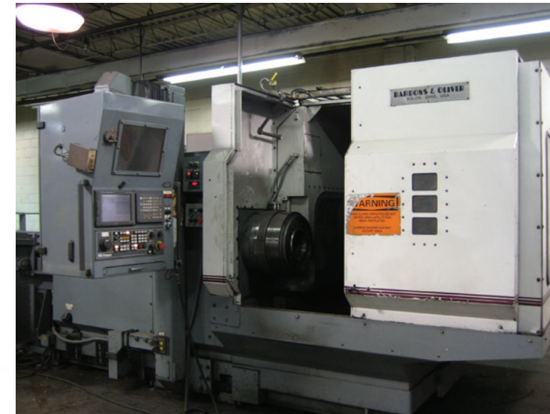
Our big bore lathes can finish-machine centrifugal castings up to 8" diameter.
